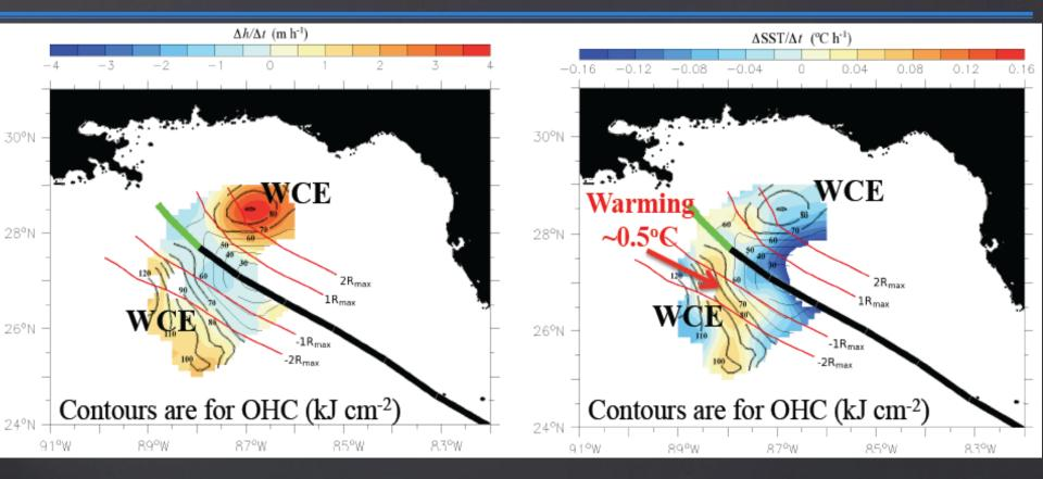
In- storm (12 h interval) Ocean Mixed layer (OML) deepening; h is OML depth.
