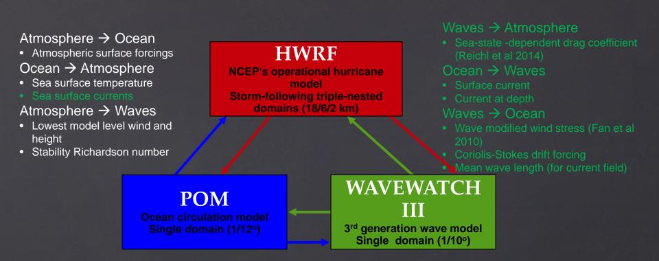
Three-way coupled atmosphere-wave-ocean HWRF system. The coupling processes in black are in currently operational HWRF and the control experiment, whereas the coupling processes in green are additional coupling processes considered in the coupled experiment.
